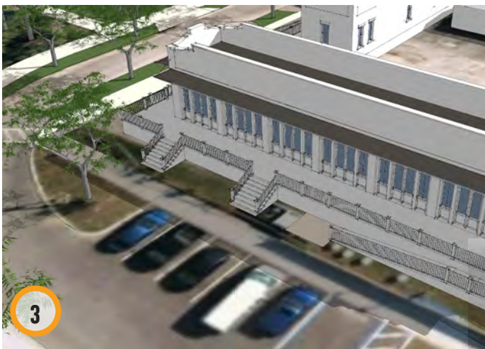
The porch frontage type can be utilized for buildings with multiple shopfronts and businesses where they share a common porch that functions as a secondary sidewalk or seating area.
