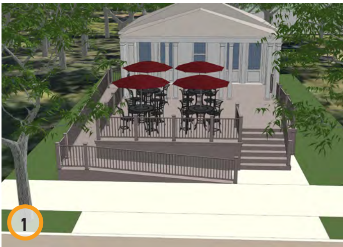
This commercial building is set back from the street with an elevated deck forming the street wall. Both steps and an ADA ramp are provided for access to the business.
