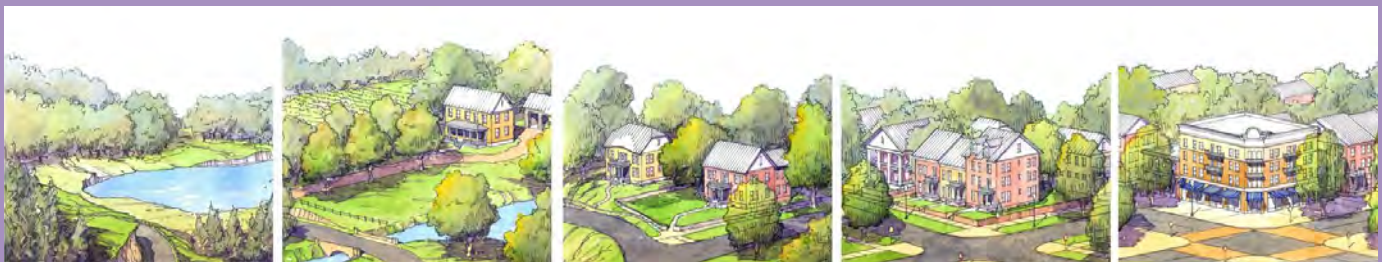
The Transect is a planning and zoning tool that organizes zones in a continuum from rural to urban, referred to as T1, T2, T3, T4-R, T4-O, and T5.
