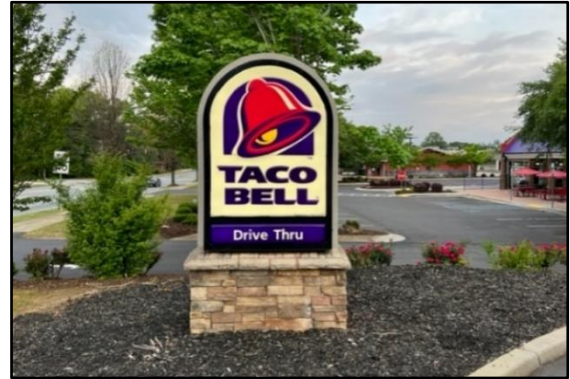
BASE WIDTH: 5'; BASE HEIGHT: 2' 6" SIGN WIDTH: 4'; SIGN HEIGHT: 6' TOTAL SIGN AREA: = 24 sf.
